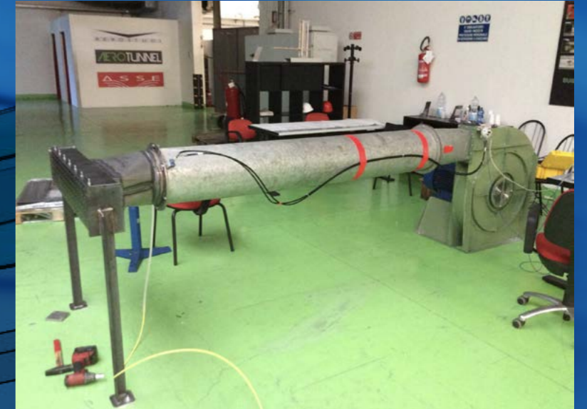
Example: test rig for aerodynamic noise measurement
